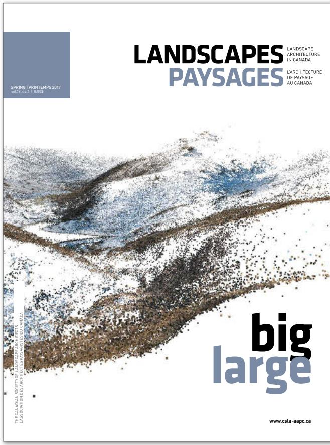
**03** From Jason Hare at Winnipeg's FABLab: Digitizing landscapes using point cloud construction – aerial images are captured by a small UAV (drone), and ultimately reconstructed into a three dimensional digital model of a landscape, consisting of millions of points.
